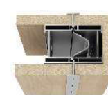
MAW110 STARTING NODE CONNECTION WITH A PANEL
